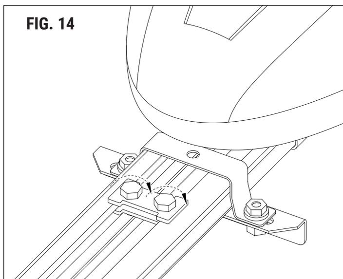
**TENSIONE CINGHIA • BELT TENSION • RIEMENSPANNUNG
